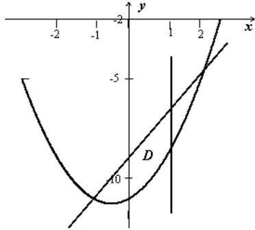
$$S(D) = \int_{-1}^1 [(2x - 9) - (x^2 + x - 11)] dx = \int_{-1}^1 (2 - x^2 + x) dx = \left( 2x - \frac{x^3}{3} + \frac{x^2}{2} \right) \Big|_{-1}^1 = \left( 2 - \frac{1}{3} + \frac{1}{2} \right) - \left( -2 + \frac{1}{3} + \frac{1}{2} \right) = \frac{10}{3}.$$
