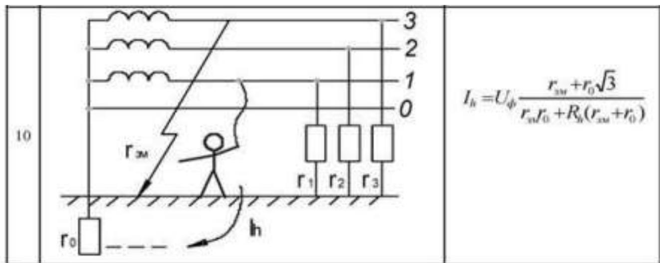
$$I_h = U_\phi \frac{r_{3M} + r_0 \sqrt{3}}{r_{3M} r_0 + R_h (r_{3M} + r_0)}$$
